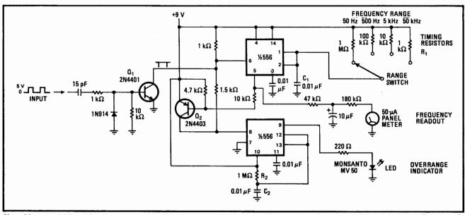
**Unambiguous.** Addition of overrange indicator to analog frequency meter warns when switch is set to wrong frequency range. Transistor Q<sub>2</sub> allows input signal to trigger LED monostable whenever input frequency is greater than meter range. Inexpensive and reliable circuit shown is useful from near dc to well over 20 kHz.
